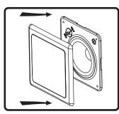
**11.** Align tabs on snap-fit grille with slots in baffle, gently press grille into place.
